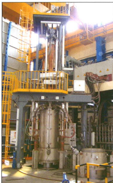
ESR Furnace with Inert atmosphere
